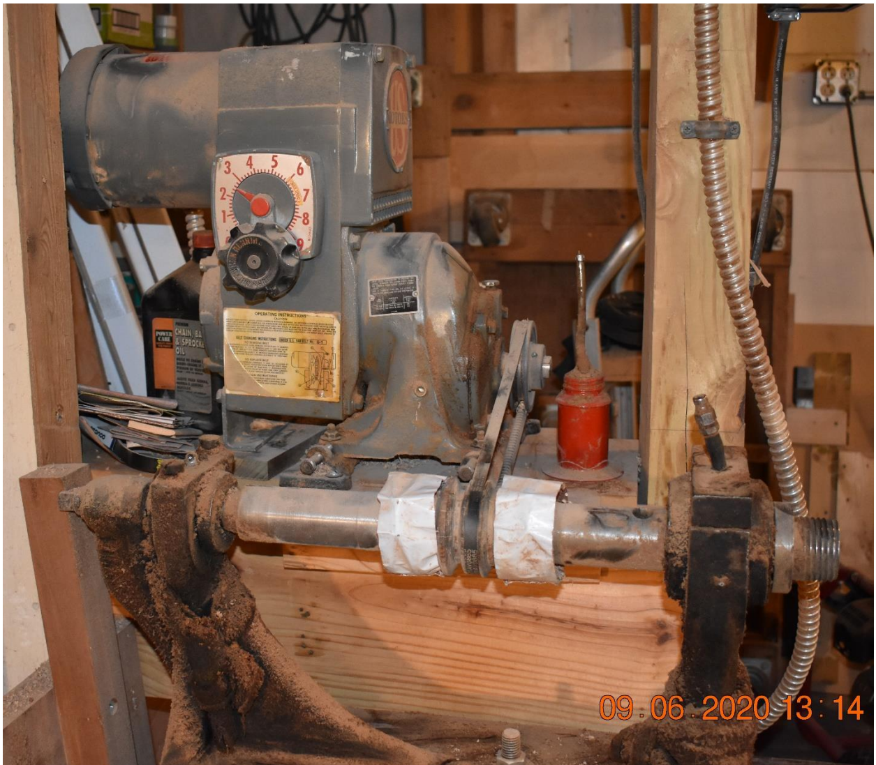
1 H.P. 3 Phase Motor - Adjustable Speed Pulley
