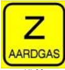
KL03 aardgasleiding in watergang of kanaal
