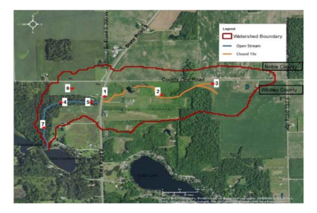
• The first priority was State Road (SR) 9 Ditch Stabilization, which according to the engineers will reduce sediment loading by 11 tons. Thanks to the persistent efforts of Denise McCann INDOT finally broke up the concrete lined ditch that was undermined on both the east and west sides of SR 9 and added rip-rock along with grass over-seeding. (Site #1)
