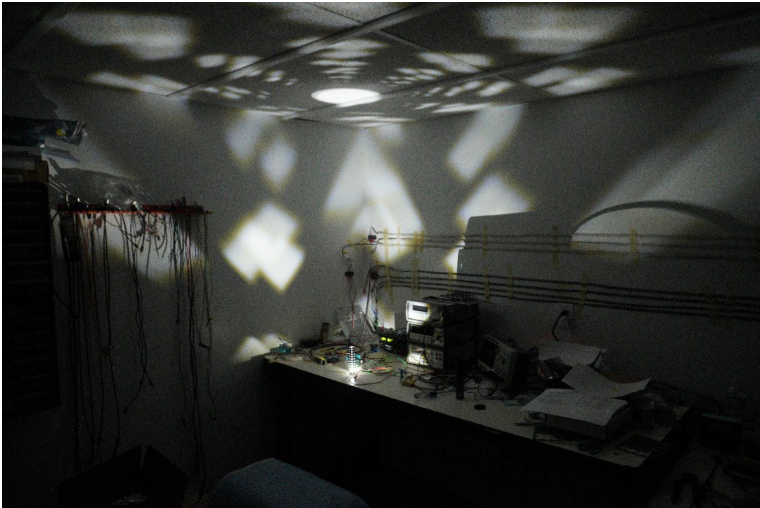
Figure 6, Lab testing the raw board inside a light diffuser with diamond holes
