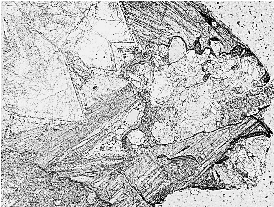
NRS Sample #2, NRS2/S2 OKS_010.jpg/PPL/FOV = 27 x 46 mm SILICEOUS FAULT BRECCIA showing typical appearance of coarsely crystalline euhedral quartz and silicified carbonate crystals in a sample not affected by ductile deformation.
