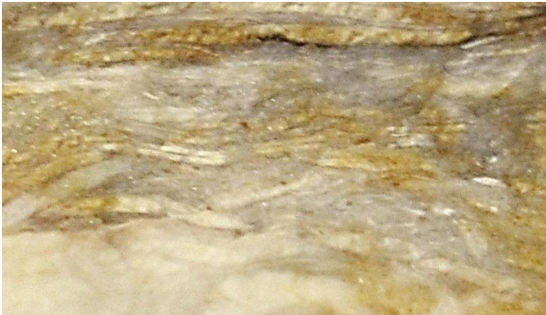
Figure 7. Mitchell quarry site chert: top image , weathered surface of a chert-like-stone sample from the Mitchell Plantation quarry site in Sussex County, Virginia; bottom image , magnified view of an old fracture surface from the sample shown in image 1, which shows silicified calcite crystals in a chalcedony and micro-grain quartz structure. (NRS collection; scale is cm.)
