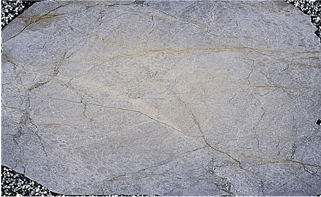
NRS Sample #3, NRS3/S1 0KS_013.jpg/XPL/FOV = 27 x 46 mm CHLORITE-SERICITE-QUARTZ SCHIST showing typical appearance.
