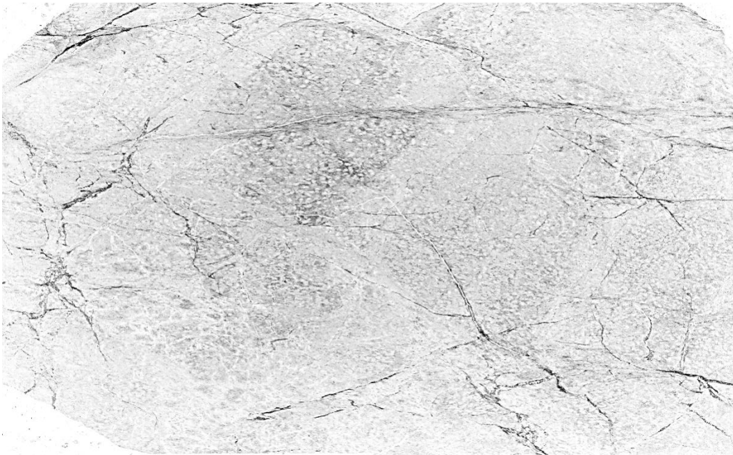
NRS Sample #3, NRS3/S1 0KS_013.jpg/PPL/FOV = 27 x 46 mm CHLORITE-SERICITE-QUARTZ SCHIST showing typical appearance.
