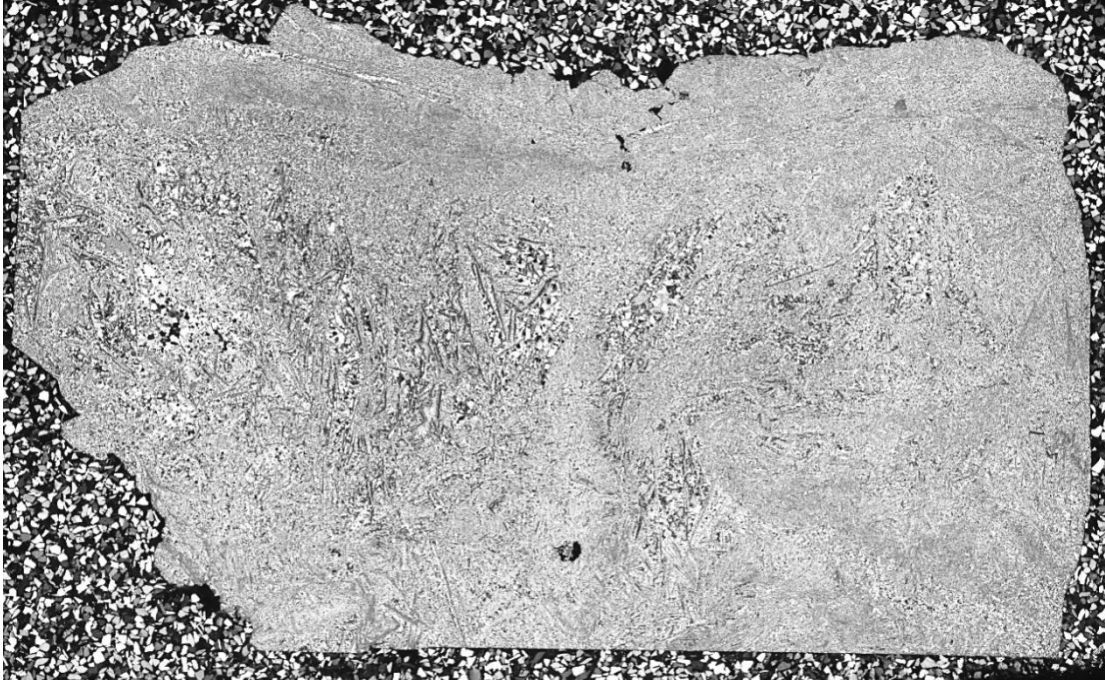
NRS Sample #6, NRS4/S1 0KS_023.jpg/XPL/FOV = 27 x 46 mm SILICEOUS SCHIST showing typical appearance of coarser grained quartz and elongate silicified calcite crystals rotated parallel by ductile deformation.
