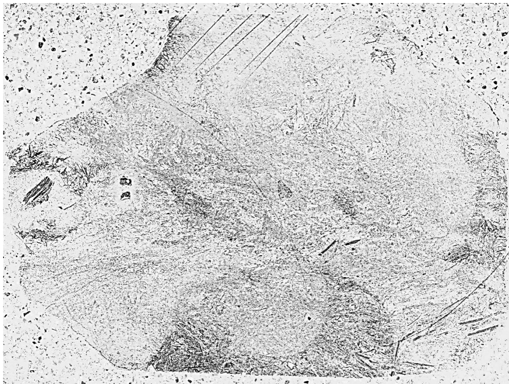
NRS Sample #5, NRS4/S1 0KS_022.jpg/PPL/FOV = 27 x 46 mm SILICEOUS SCHIST showing typical appearance of coarser grained quartz and elongate silicified calcite crystals rotated parallel by ductile deformation.
