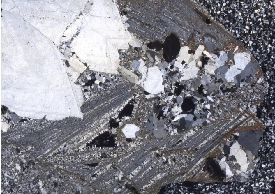
NRS Sample #2, NRS2/S2 OKS_009.jpg/XPL/FOV = 27 x 46 mm SILICEOUS FAULT BRECCIA showing typical appearance of coarsely crystalline euhedral quartz and silicified carbonate crystals in a sample not affected by ductile deformation.
