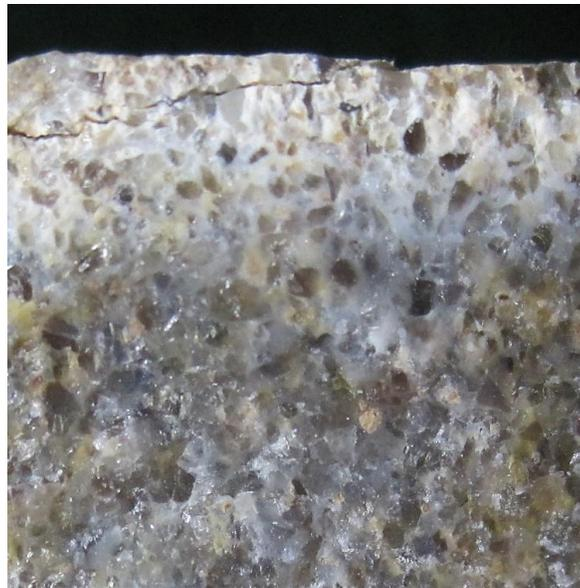
**Figure 2.** Typical Nanjemoy or Stafford County orthoquartzite with fine to large sand grain size and lithic fragments, from Stafford County, Virginia along Potomac Creek.
