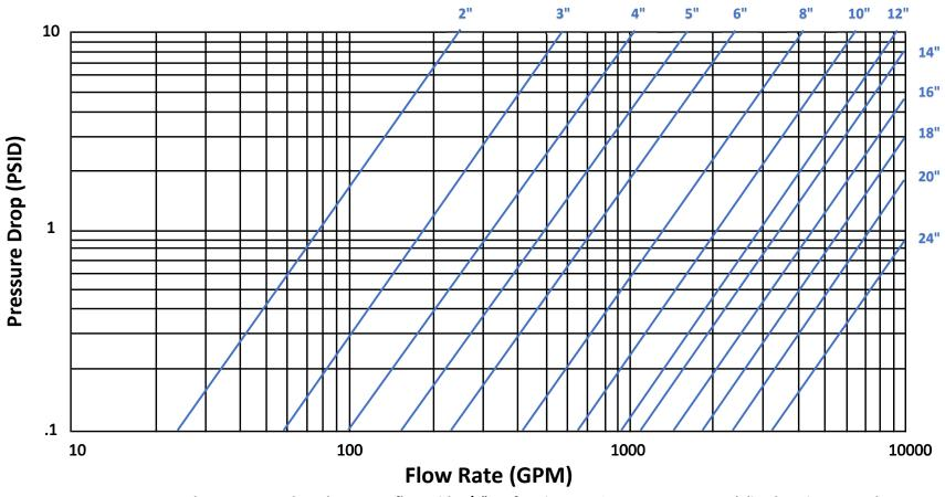
Notes: Pressure drop curves are based on water flow with 1/8" perforations, 40% open area. For mesh lined strainers, see the "MESH CORRECTION CHART"
