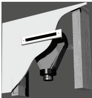
Figure 2. Typical Wall Installation, 90° Outlet
