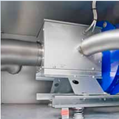
encapsulated motor with separate ventilation
