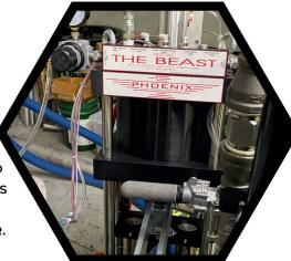
~ WITH AN AVAILABLE *5:1 PUMP*, THIS SYSTEM HAS THE ABILITY TO DELIVER UP TO 150 LBS PER MINUTE OF COMPLETELY CATALYZED POLYMER MATERIAL.
