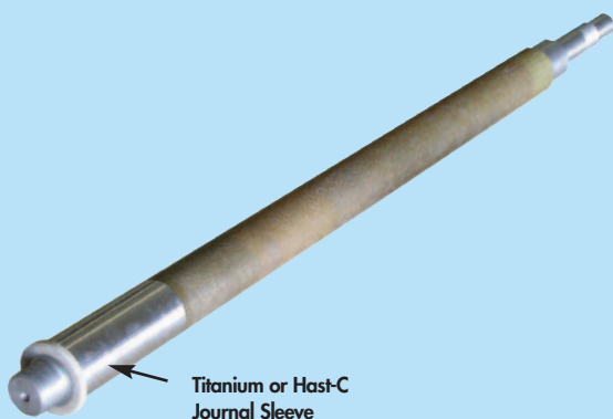
Figure 2 - Typical fiberglass-wrapped 303SS shaft. The shaft is available with either a Titanium or Hastelloy-C Journal Sleeve for the lower sleeve bearing located in the pump cover.
