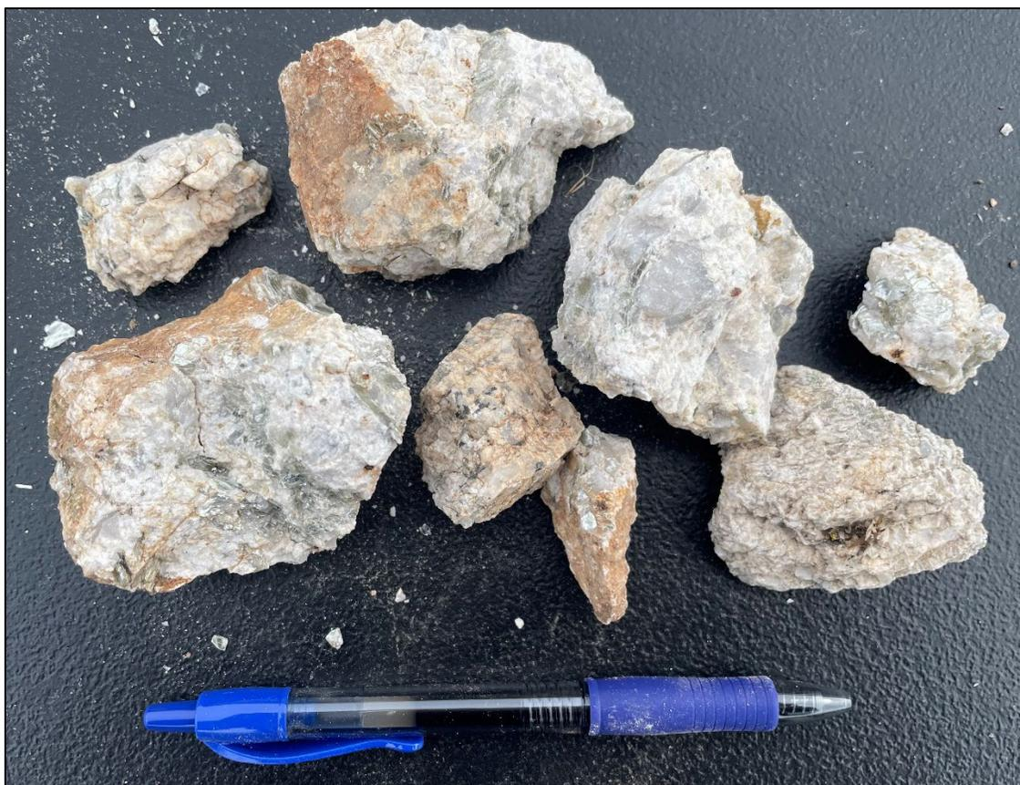
Figure 9: Sample MO-015. Sample pegmatite from historical workings. Constituent mineralogy includes quartz, albite, accessory muscovite, and rare black tourmaline. Sample MO-015 is representative of the average mineralogy in the gathered pegmatite samples.
