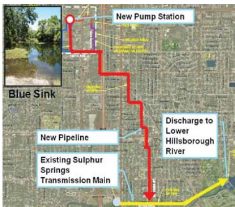
Figure 19. Proposed Blue Sink diversion facilities.
