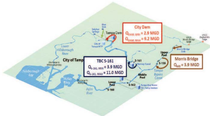
Figure 23. Planned infrastructure at TBC S-161 and the Hillsborough River Dam to implement Tampa Bypass Canal diversions.
