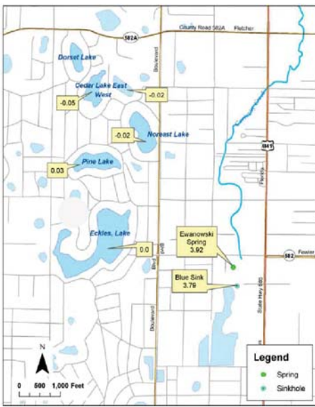
Figure 20. Lake drawdown (in ft) during the Blue Sink Pump Test.
