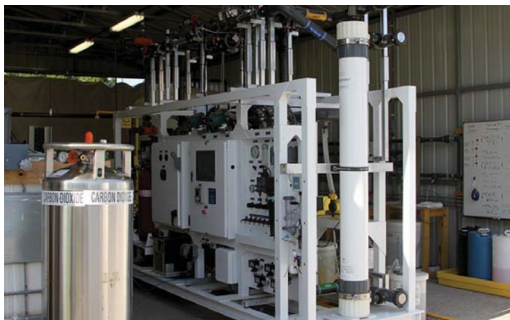
The ultrafiltration component of the pilot treatment plant. Ultrafiltration removes suspended solids, bacteria, and microconstituents.
