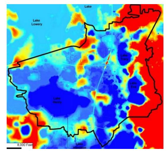
LiDAR Based Digital Elevation Model
