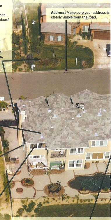
**Walls:** Wood products, such as boards, panels or shingles, are common siding materials. However, they are combustible and not good choices for fire-prone areas.
