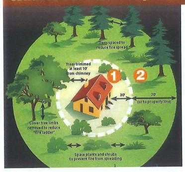
Defensible space is the required space between a structure and the wildland area that, under normal conditions, creates a sufficient buffer to slow or halt the spread of wildfire to a structure. It protects the home from igniting due to direct flame or radiant heat. Defensible space is essential for structure survivability during wildfire conditions.
