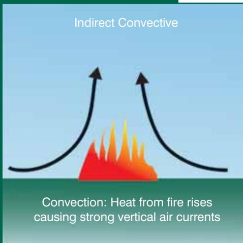
Figure 2-7: Convective lifting
