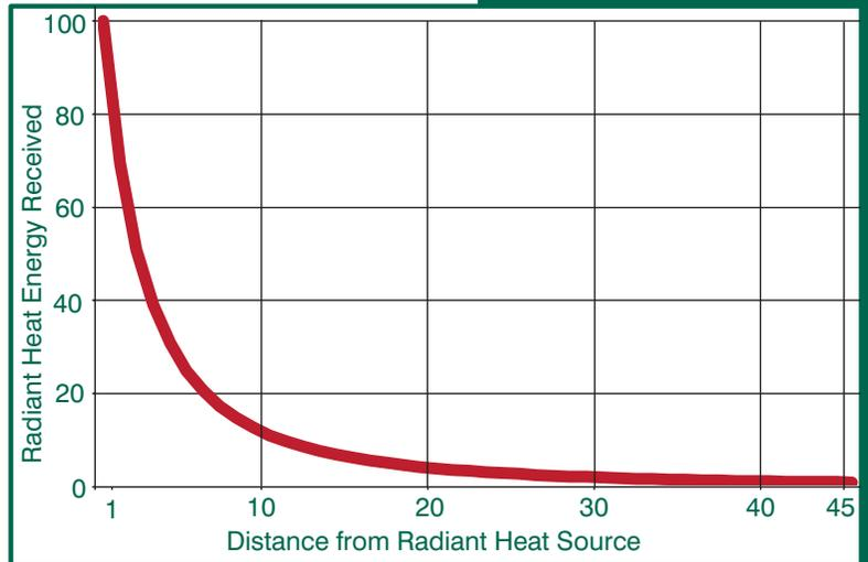
Figure 2-4: Radiant energy decreases with increased distance
