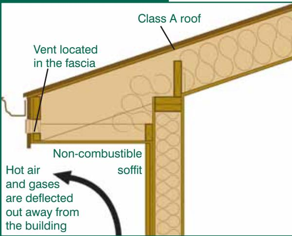
Figure 4-9: Fully enclosed soffit with isolated vent
