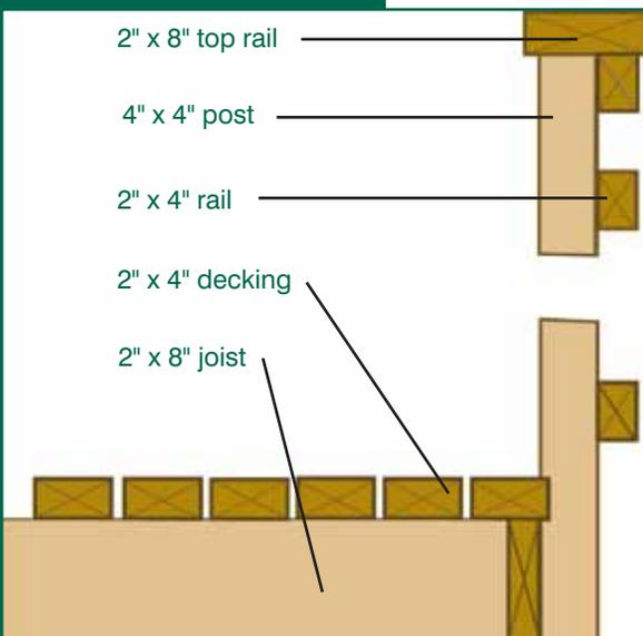
Figure 4-11: Conventional deck construction detail
