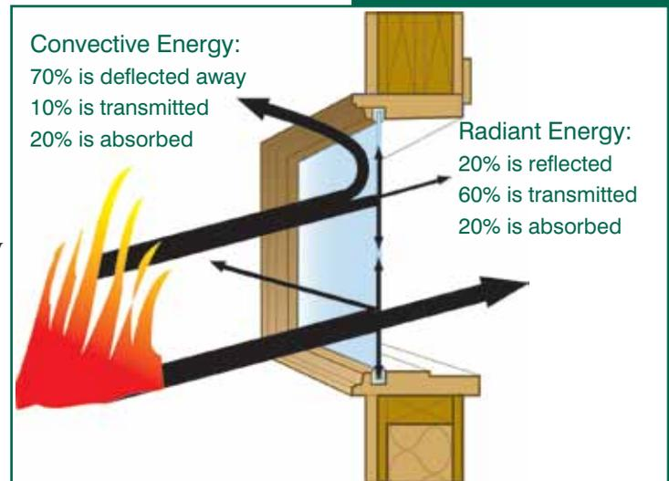
Figure 5-10: Energy transmission, conventional glass
