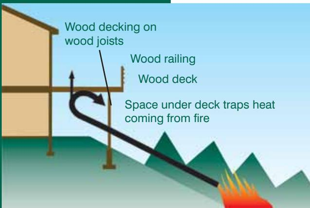
Figure 4-10: Conventional deck in a fire
