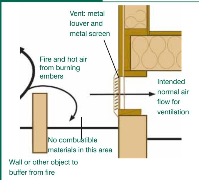
Figure 4-5: Crawl-space ventilation
