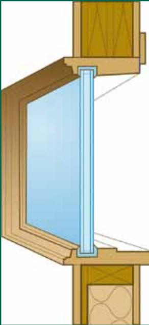
Figure 5-12: Thermopane window
