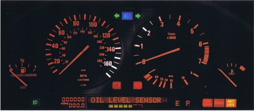
All instruments are directly in the driver's line of sight with large analog dials for primary information such as road speed and engine speed, and digital displays for mileage and secondary information such as the Check/Control system.
