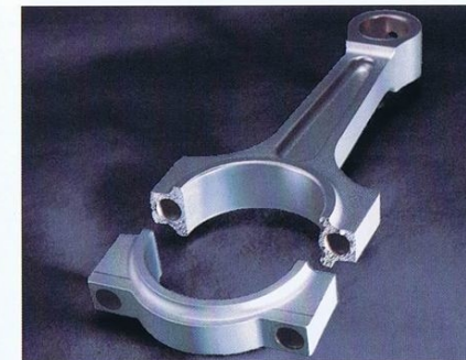
Just one of many new quality innovations in the 8-cylinder engine: for the first time in a BMW production engine, sintered connecting rods were designed for perfect fit. The result: 17% weight reduction compared to standard rods, yet stronger and finely balanced for smooth engine operation at all speeds. Broken apart in a specific fracture pattern at a predetermined point, both parts form an extremely stable, centrally aligned unit when mounted to the crankshaft. Another example of BMW's quest for quality.
