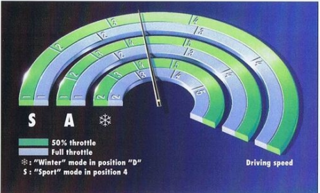
Five-speed automatic transmission offers a choice of shift modes — Automatic and Winter — allowing the driver greater control of the driving experience, as well as efficiency of operation. Shifting from "D" to "4" allows the option of sports acceleration for dynamic driving.
