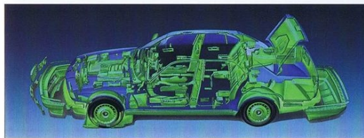
Today about 75-80% of all materials and components of a BMW can be recycled. And BMW's objective is to make our cars fully recyclable. The illustration presents the recyclable parts of the 7-Series models.
