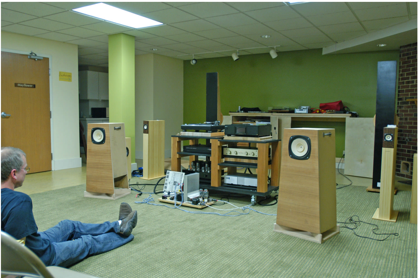
Howard Grim's high efficiency folded horn design.
