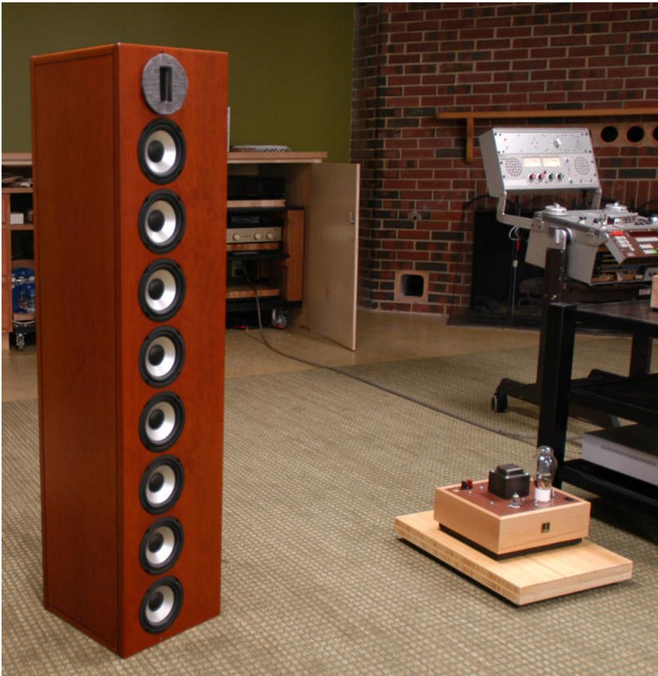
The system consisted of a Nagra T real-to-real tape machine feeding a prototype low impedance line stage and a pair of 8WPC Paramount single ended amps using 300B tubes and the discontinued 96dB sensitive Straight 8 loudspeakers.
