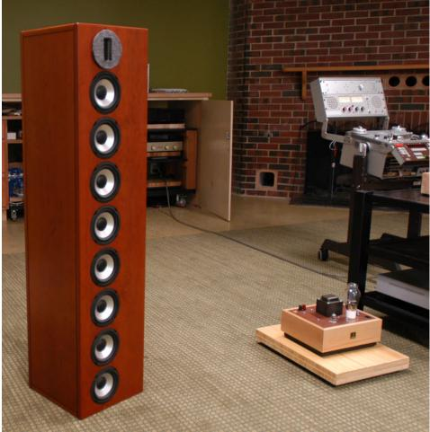
The system consisted of a Nagra T real-to-real tape machine feeding a prototype low impedance line stage and a pair of 8WPC Paramount single ended amps using 300B tubes and the discontinued 96dB sensitive Straight 8 loudspeakers.
