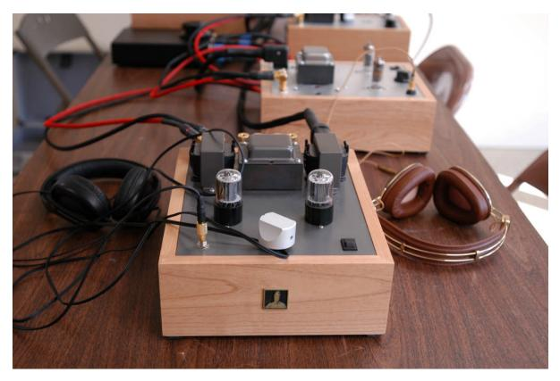
S.E.X. amp (Single Ended eXperimenter's) kit 2.1 for headphones and high efficiency speakers sells for \$499 in kit form.
