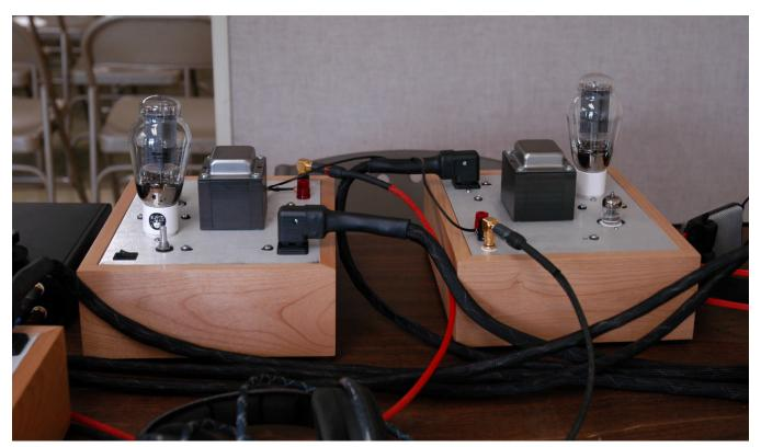
A pair of the 8WPC Paramount single ended mono amps using 300B tubes driving the discontinued AKG K1000 headphones. The pair in kit for sells for only \$1,549, the ultra-high-end for a pittance.
