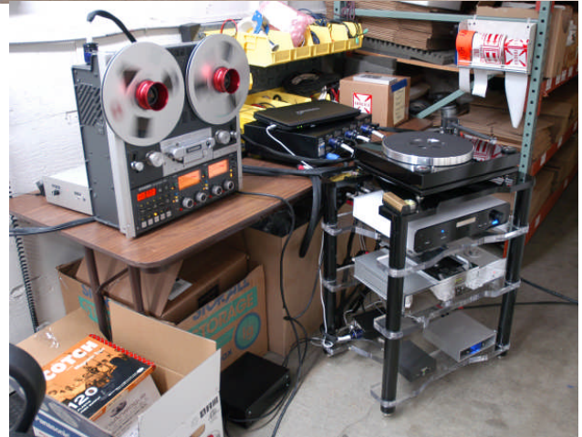
Tape Meister Ki Choi provided his Studer A810 1/4" tape machine and stunning master tapes. Gary spun vinyl on his modified Roksan Xerxes turntable with Magic Magic Diamond cartridge. Everything running through Gary's preamp with built-in phono stage.
