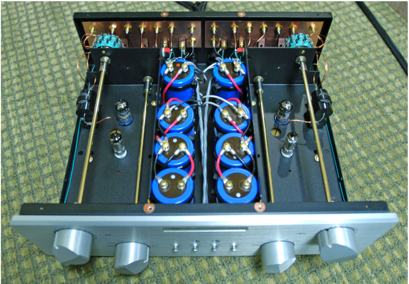
The interior view of the First Sound Presence Deluxe preamplifier shows the true dual mono layout, stepped attenuator volume controls and the massive capacitor storage.
