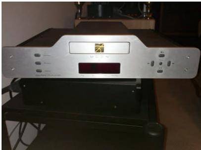
player has internal upsampling to 24-bit/352.Khz level of resolution, and a "very accurate 50PPM digital clocking system" (quoted from the manual).
