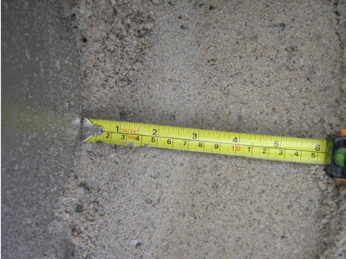
Natural gravel development up to 12 cm from well screen
