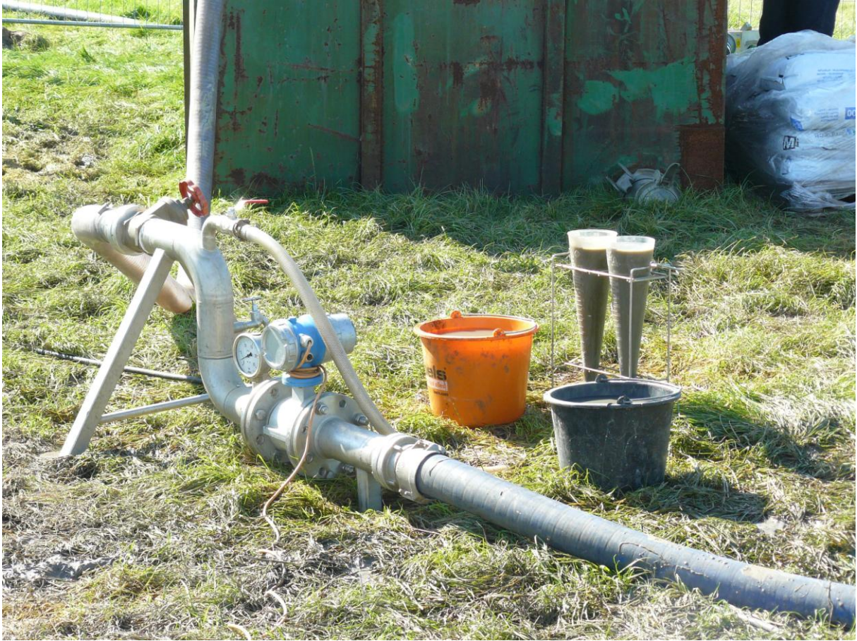
Measurement of extracted solids and taking samples
