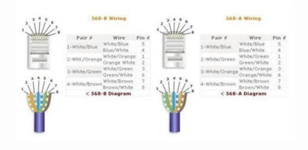
Most simple Ethernet cables I've purchased seem to use the T-568B system on both ends. For a crossover cable, use T-568B system, so I used it on both ends of the cable. For clarity and ease of viewing, at the end of this answer I have provided some rules that I follow and which you can adapt yourself as long as you follow the same wire color order.
