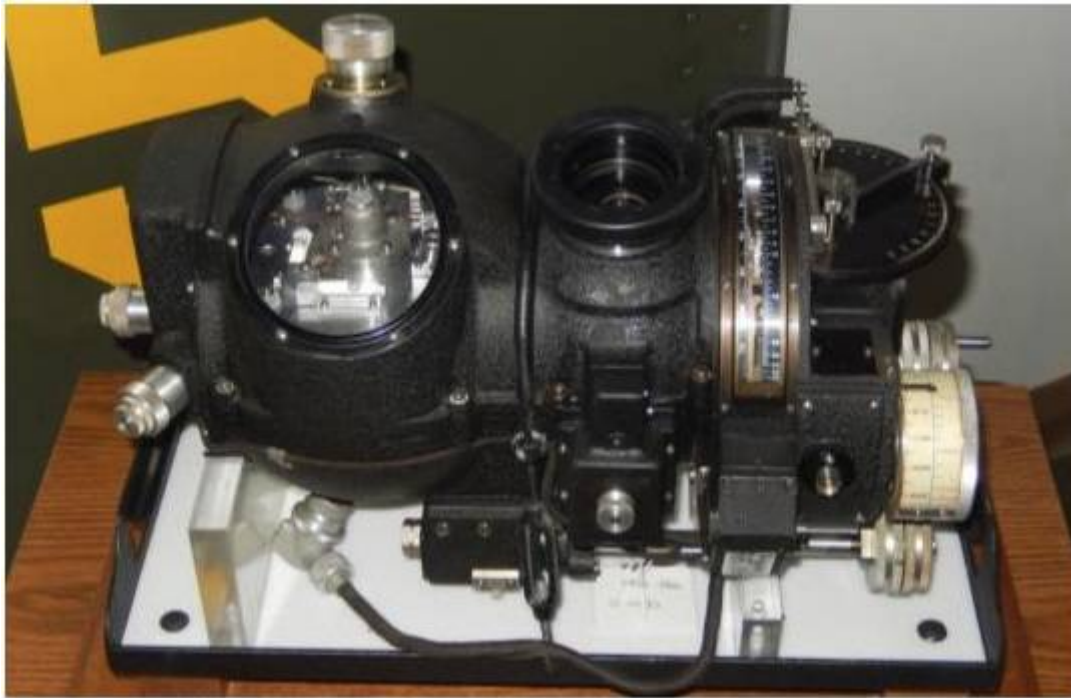
Norden Bombsight, used in the B-17, B-24 and B-29 bombers in WWII
