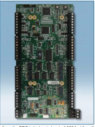
When a card's record is not found in the DDC database, the card data is passed to the NLC for the access control decision. If communication between the DDC and NLC is disrupted, the DDC continues to make access decisions for its 20,000 cardholders. Up to 512 events are stored at the DDC and passed to the NLC when communication is restored.
