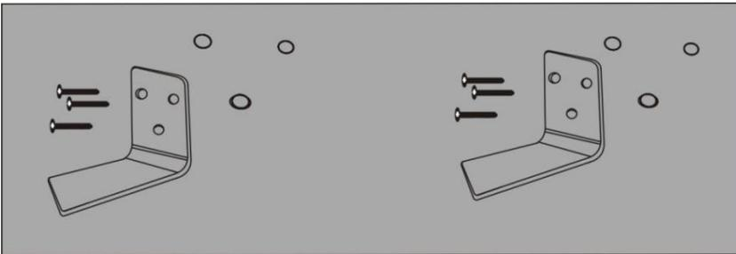
IV. Before fixing the heater, make sure the rocker power switch on the right side and then fixed the bracket to the heater using four M6\*14 screws and butterfly nuts.
