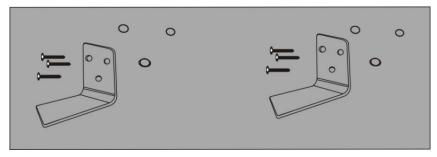
IV. Before fixing the heater, make sure the rocker power switch on the right side and then fixed the bracket to the heater using four M6\*14 screws and butterfly nuts.
