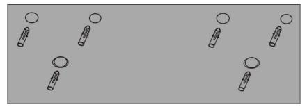
III. Fix the bracket using six ST4\*35 screws and make sure the installation points are fixed securely.
