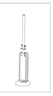
STEP 3 Place the tank housing on the stand.
