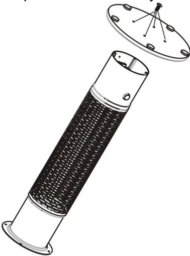
Step 2: Fix the stainless steel table and product together with 4pcsM5\*14MM screws
