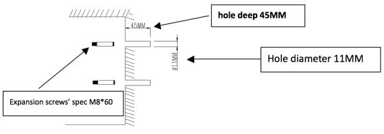
Step 4: Fix adjusting bracket into wall with expansion screws.
