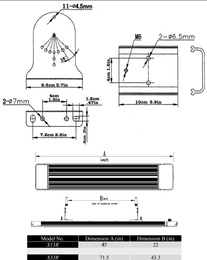
Step 1: Installation of adjusting bracket and sliding bracket.
