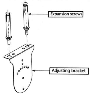
Step 5: Installation of two adjusting brackets. Make sure to lock brackets tightly by using the butterfly hand screw.
