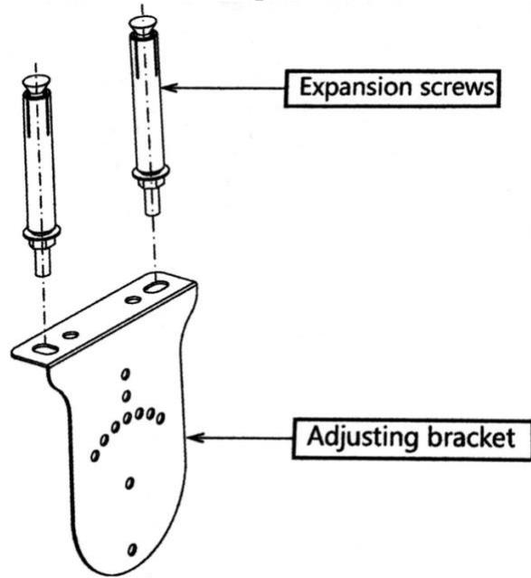
Step 5: Installation of two adjusting brackets. Make sure to lock brackets tightly by using the butterfly hand screw.
