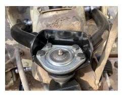
Lowers should be installed as pictured below, the ball joint will go approximatley  $\%^{\prime\prime}$  deep when pressed from the bottom
