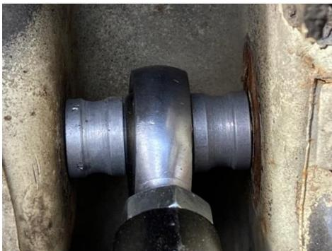
Proper upper control arm spacer install
