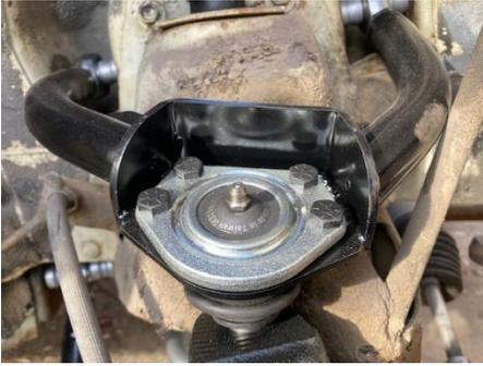
Lowers should be installed as pictured below, the ball joint will go approximately ½" deep when pressed from the bottom
