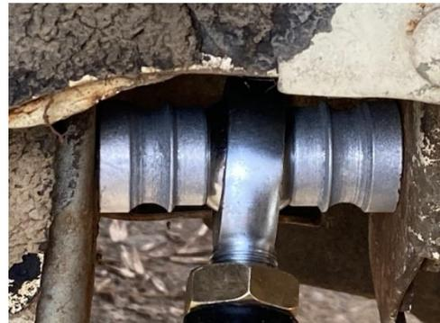
Proper lower control arm spacer install
