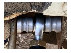
Proper lower control arm spacer install
