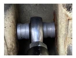
Proper upper control arm spacer install
