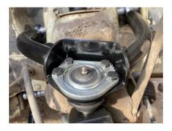
Lowers should be installed as pictured below, the ball joint will go approximatley % deep when pressed from the bottom
