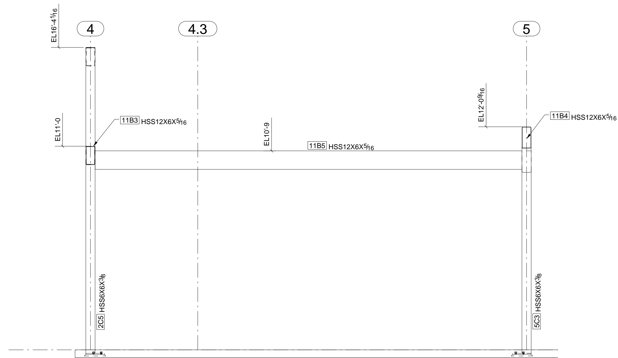
K - K ~ELEVATION VIEW GRID LINE A
