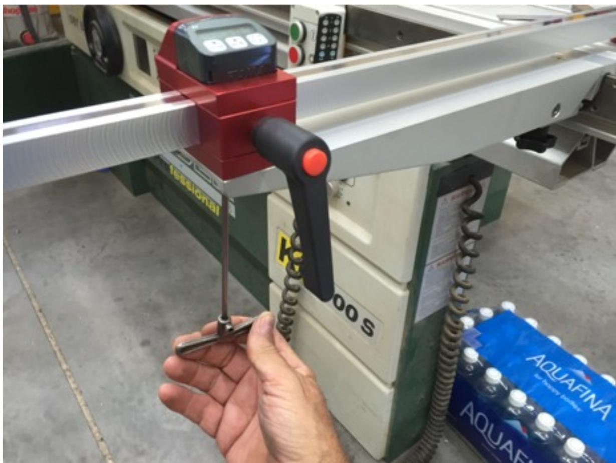
Installation is now complete, the next section details the procedures for setting the zero and explains how to use the buttons on the DRO. You will also receive the manual from Fiana, it can be slightly confusing though, so we will detail the procedures to set options on the unit.
