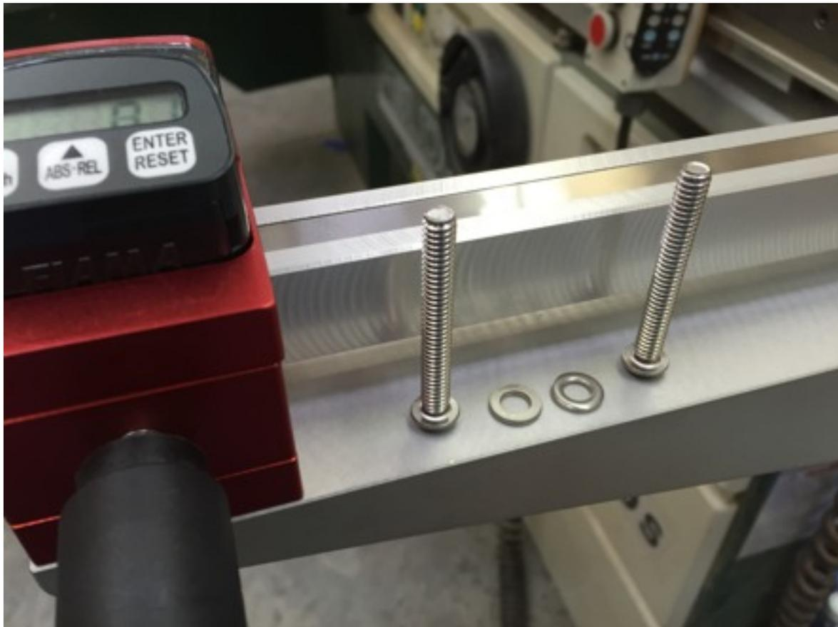
Tighten all four bolts, there is a small amount of tolerance in the bolt holes, so you may want to put a small square across the C-channel and square up the rear block as you tighten it.
