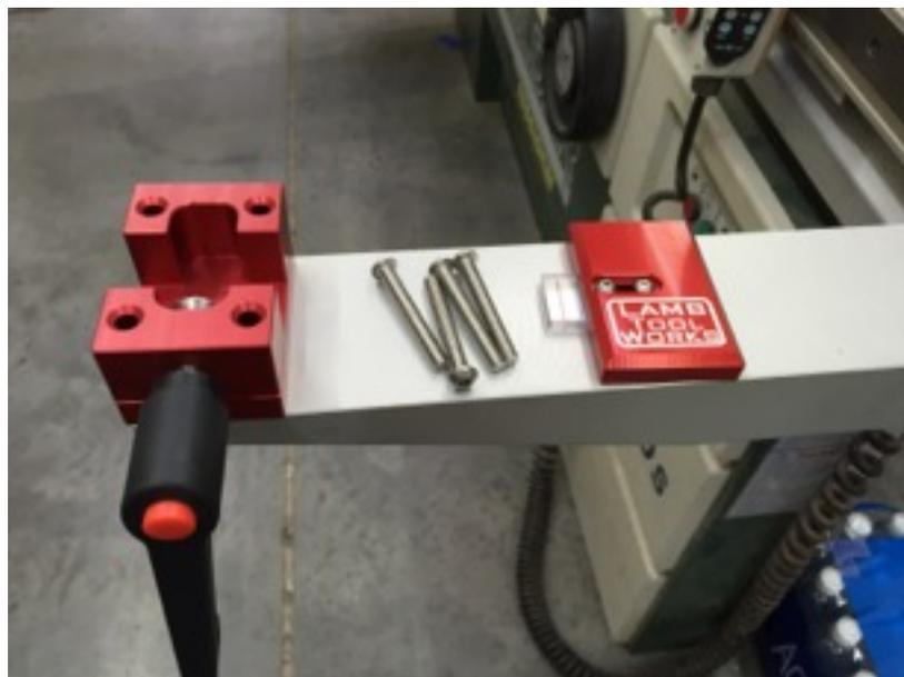
We now need to remove the end stop from the measuring rod and transfer it to the new rod supplied with the kit. You will need to use the 1/8" ball hex driver to get at the angle to remove the 10-32 screw holding the end stop on, you may need a cheater on the short end of the wrench to break it loose. After you remove it, just re-install it on the end of the new rod that has the magnetic banding in it.
