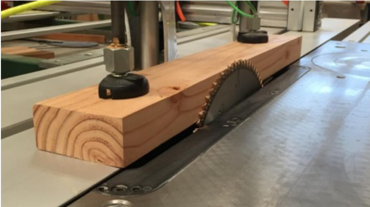
Next, clamp a scrap piece of 1x2 to the fresh cut edge, this gives you a surface to set the stop against and get a perfect zero reading.
