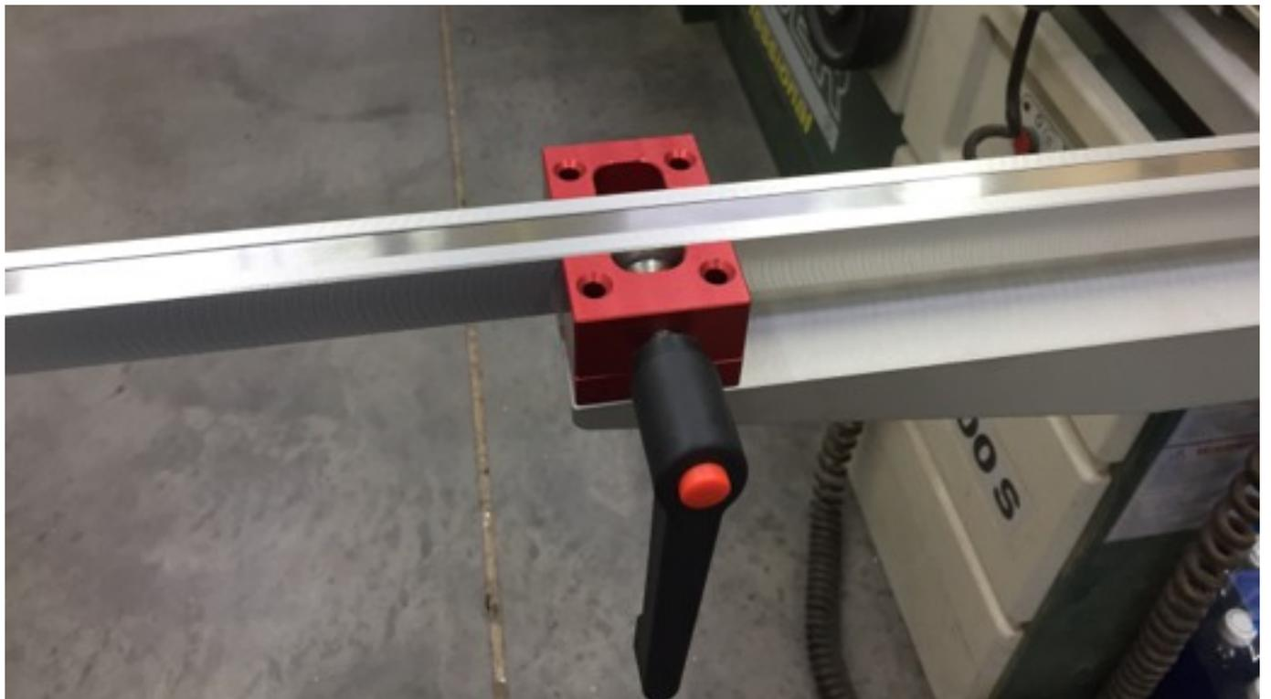
Now, install the new rear cap with the installed Fiamsa DRO unit.
