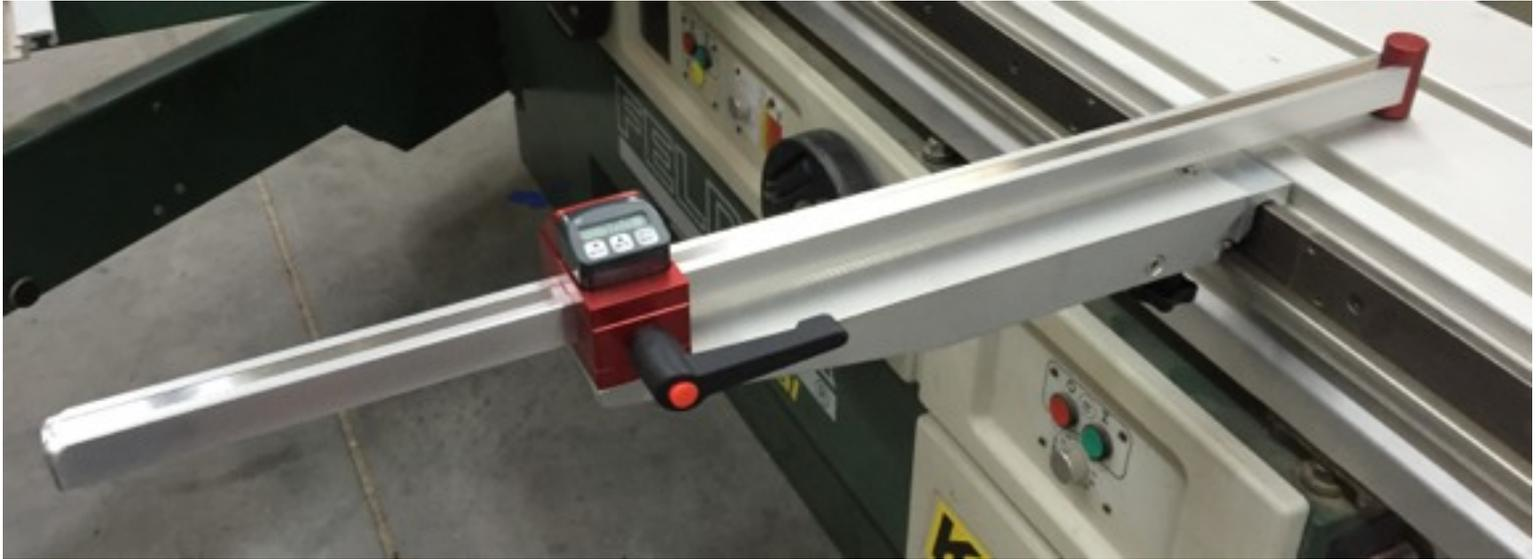
This document will walk you through upgrading your existing Parallel Fence with a Digital Read Out option. The process is fairly simple and you will need two tools, a 1/8" ball end hex key, and a 5/32 hex key (allen wrench).
