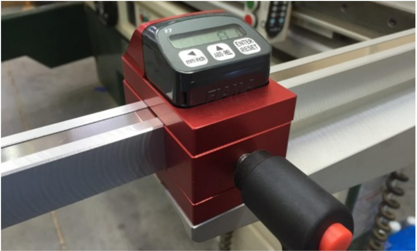
Using the long 1/4-20 Button Head Cap Screws you removed, install the supplied washers onto two of them and install them on the side closest to you in the picture below, the short side closest to the DRO. It would be wise to use some grease or anti-seize on the ends of the threads of the bolts.
