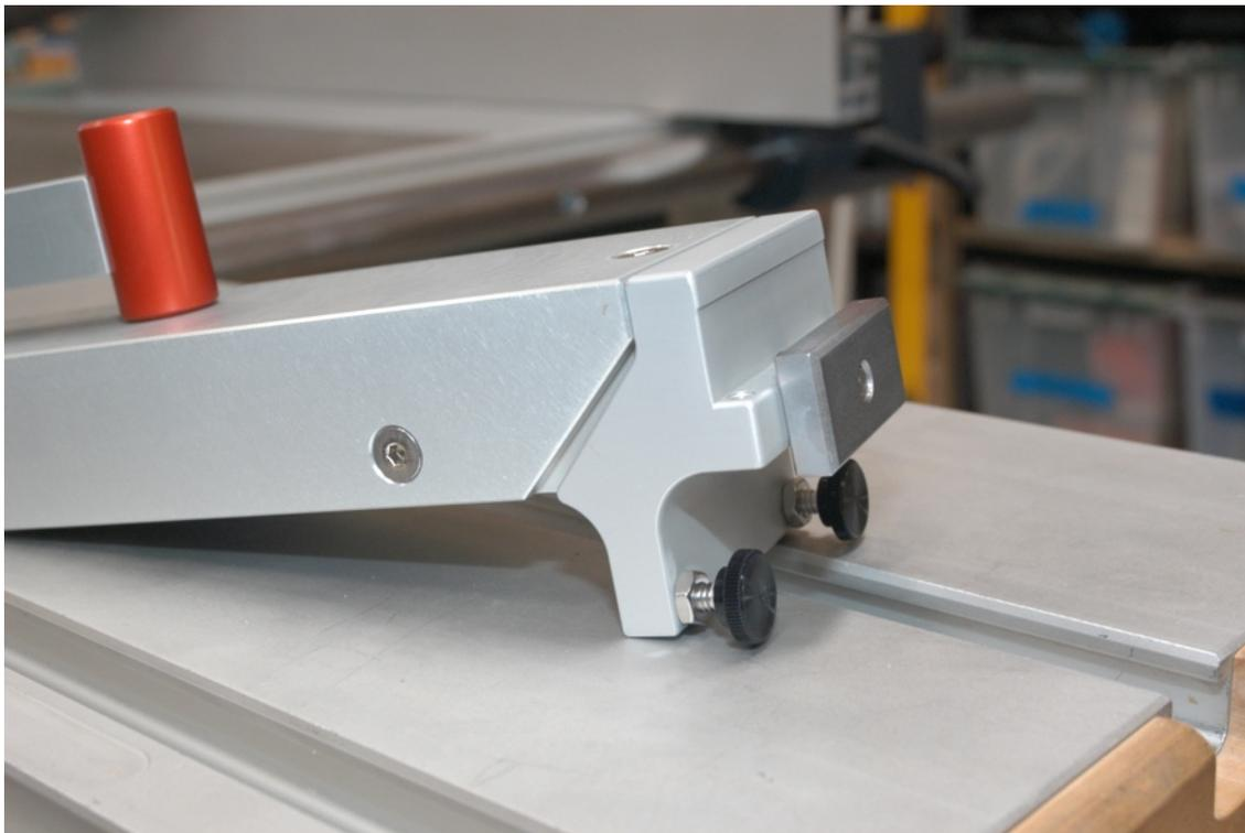
This is what the clamp will look like out of the box. The thru bolt will be holding the t-slot nut tight to the mounting head. Note that all the hardware is stainless steel, but the t-slot nut is not so you might want to oil or wax the nut to prevent rust if you live in a humid environment.
