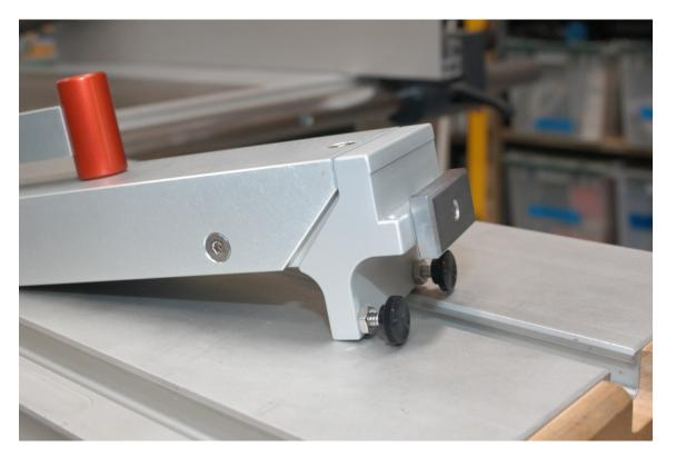
This is what the clamp will look like out of the box. The thru bolt will be holding the t-slot nut tight to the mounting head Note that all the hardware is stainless steel, but the t-slot nut is not so you might want to oil or wax the nut to prevent rust if you live in a humid environment.
