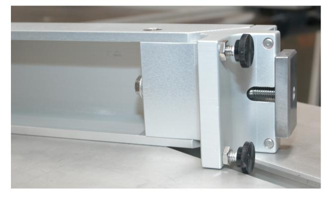
Remove the t-nut and slide it into the slot on your slider, the larger chamfers go towards your Minimax. The thru bolt is held captive in the mounting head by a keeper, so no need to worry about loosing parts. You can now hold the head onto the machine, check to see if the jacks screws need adjusting to level the pitch of the parallel fence. Loosen and adjust the jack screws as necessary to get the top of the fence level. Note, it might be slightly below the surface, that is adjusted next.
