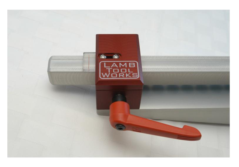
Now it is time to set the scale. With the parallel fence now mounted on your slider, extend the stop and measuring rod until the stop is at the blade. Use a piece of paper between the blade and the stop so as to not scratch the stop, but get the paper to be sticking between the high spot on the carbide tips and the stop. This is essentially "0".
