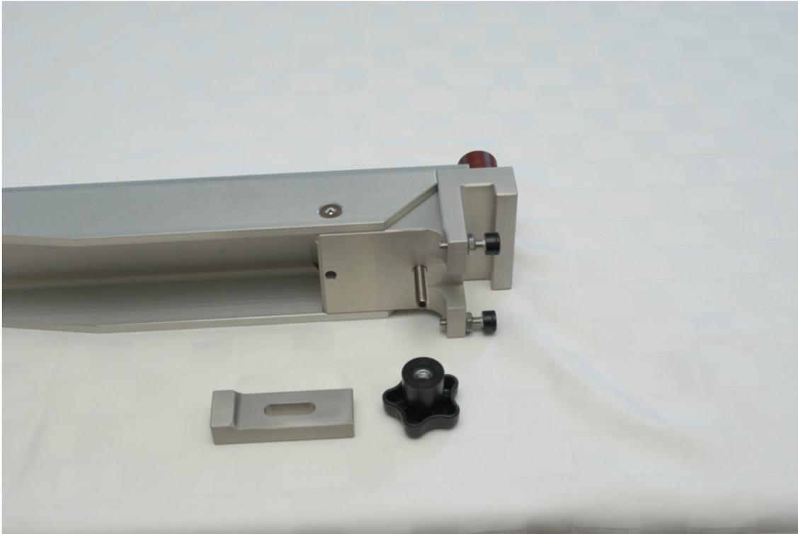
Remove the clamp assembly and while it is off, let's go to the machine and set the parallel fence to be level to the slider. You will need to insert the parallel fence from the end of the slider. Hang the hook portion over the channel portion, the black support screws can now be adjusted to set the fence parallel to the slider. Use a 7/16" wrench to unlock/lock the nuts.
