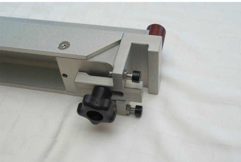
This is the clamped orientation, the clamp extends forward and pulls the fence firmly down onto the slider.
