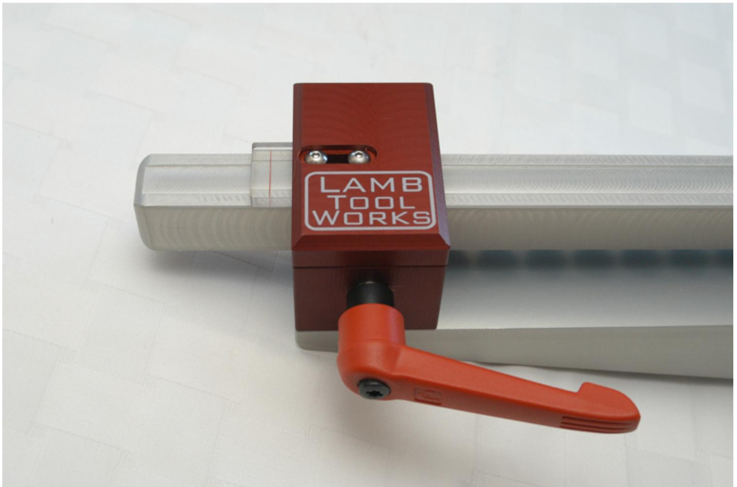
Now it is time to set the scale. With the parallel fence now mounted on your slider, extend the stop and measuring rod until the stop is at the blade. Use a piece of paper between the blade and the stop so as to not scratch the stop, but get the paper to be sticking between the high spot on the carbide tips and the stop. This is essentially “0”.
