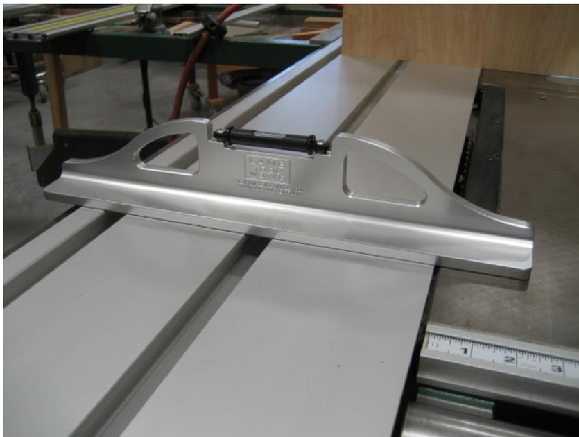
When the saw table flatness is established, you can use the same settings on the LTW level to adjust the sliding table. It is best to have your slider's bearings directly between the position of the level and the support bolts on the lower slider carriage so things are solid and you get a consistent reading.
