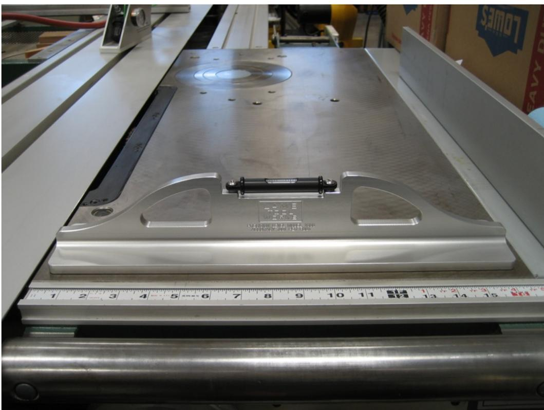
To level the cast iron top of a saw table, place the LTW level as shown to see if the machine is fairly close to level to begin with. If the bubble is to the left, then the left side of the machine is high; to the right, then the right side is high.
