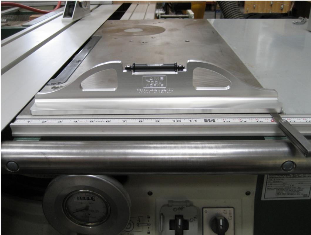
If you would prefer to leave the LTW level as set from the factory at level, you can always use feeler gages to achieve level and then transfer the feeler gages to wherever you are getting comparison readings. In this example, .042" of feeler gages were required to get a level reading. To check the rear of the table, the LTW level and the feeler gages will have to be transferred and the same distance maintained between the feeler gages and the end that is resting on the table.
