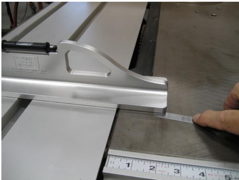
The height of the sliding table above the cast iron saw top is also easily checked by using feeler gages along the edges of the slider as shown. First in the front of the saw, then in the rear.
