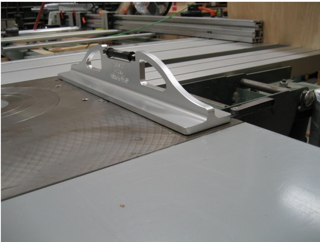
Here is the LTW level in the rear position, showing the feeler gages sticking out the back of the saw table. Care must be used to maintain the position of the shims so that you get consistent readings.
