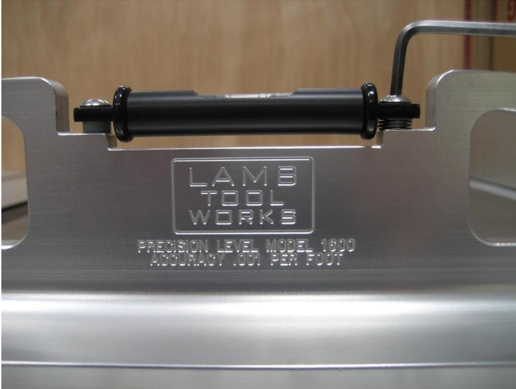
This is a close up of the vial, showing the ability to adjust it for level. One side is fixed permanently using the socket screw and a nylon washer under the vial with Loctite. **Do not adjust this side.** The right side is where adjustments for level are made, where there are a stack of spring washers between the vial and the level body. The adjusting screw is a fine pitch thread, so adjusting for level is relatively easy even though the vial is very accurate.
