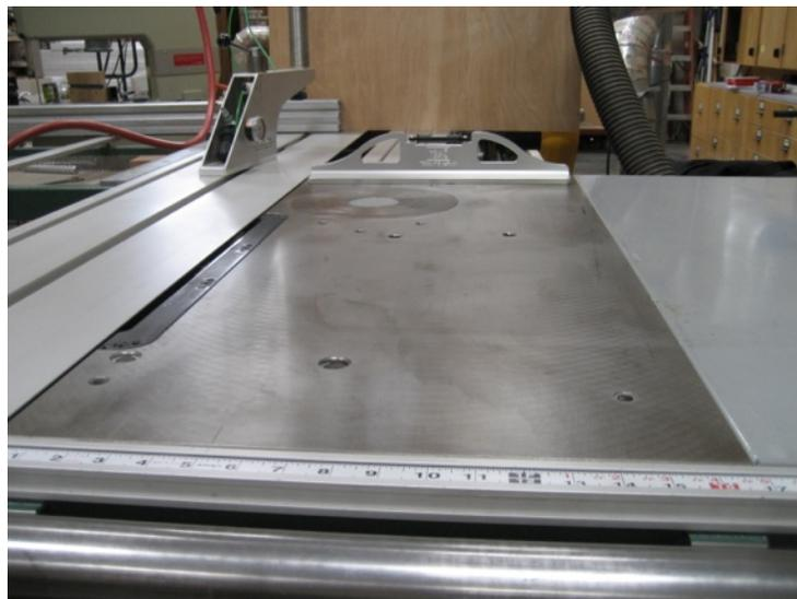
Once you have finished calibrating the LTW level, you can then slide it to the rear and see if it is still level. If you have the saw table flat, all future adjustments become a lot easier to accomplish. How adjustments to specific saws are accomplished will have to be determined by the user, as they all vary somewhat. When you have the front and rear edges in the same plane, a straight edge front to back is best to determine if there are dips or high spots in the length of the table.
