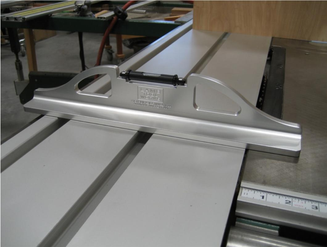
This method of using shims is probably not the best idea if you intend to use the LTW level to also adjust your slider. Because the position of the feeler gages needs to be consistent, on a narrower sliding table, the feeler gages would be off the table, or the opposite end of the level could be hanging off the table on the other side as shown in this picture. This would vary the contact points and throw off the readings of the LTW level.
