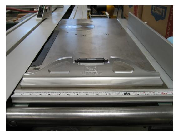
To level the cast iron top of a saw table, place the LTW level as shown to see if the machine is fairly close to level to begin with. If the bubble is to the left, then the left side of the machine is high; to the right, then the right side is high.
