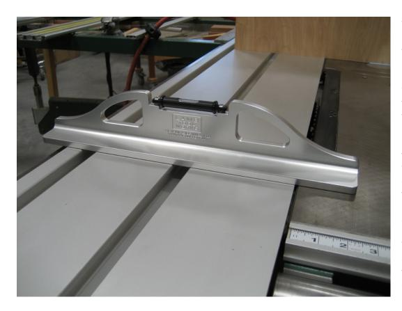
This method of using shims is probably not the best idea if you intend to use the LTW level to also adjust your slider. Because the position of the feeler gages needs to be consistent, on a narrower sliding table. the feeler gages would be off the table, or the opposite end of the level could be hanging off the table on the other side as shown in this picture. This would vary the contact points and throw off the readings of the LTW level.
