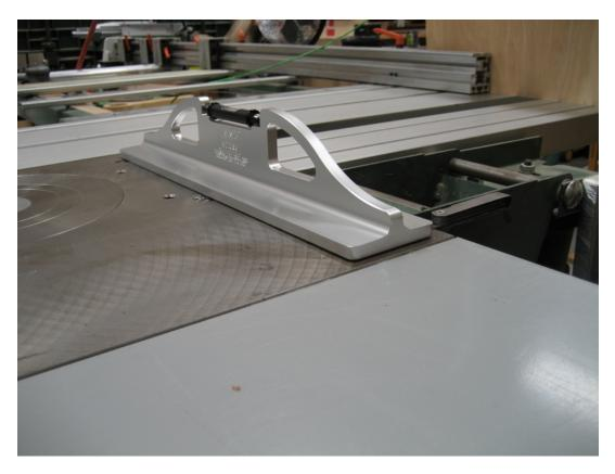
Here is the LTW level in the rear position, showing the feeler gages sticking out the back of the saw table. Care must be used to maintain the position of the shims so that you get consistent readings.
