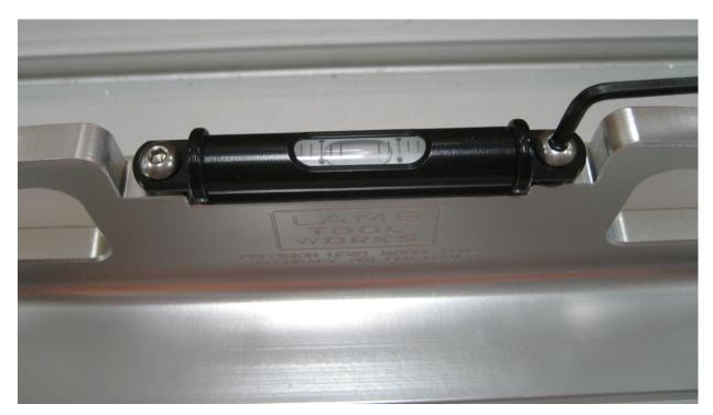
4) Spin the level 180° and the bubble will be a specific amount off to one side. Raise or lower the vial accordingly to place the bubble half way between the two readings.
