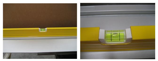
3) Place the LTW level in the same location on the slider, using the calculated stack of feeler gages if necessary. Adjust the vial to read level, remember, there is a limited amount of travel in the vial adjustment, so if the springs start to compress too much, spin the level and attempt to use the adjustment with it facing the opposite direction. Here we have adjusted the vial centered (camera angle makes it look slightly to the left).
