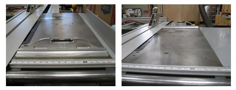
Once you have finished calibrating the LTW level, you can then slide it to the rear and see if it is still level. If you have the saw table flat, all future adjustments become a lot easier to accomplish. How adjustments to specific saws are accomplished will have to be determined by the user, as they all vary somewhat. When you have the front and rear edges in the same plane, a straight edge front to back is best to determine if there are dips or high spots in the length of the table.
