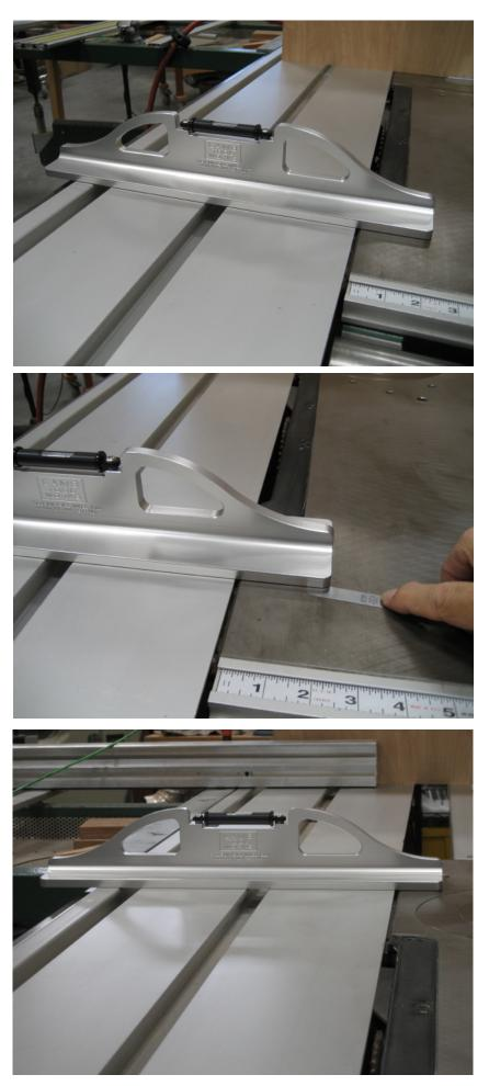
When the saw table flatness is established, you can use the same settings on the LTW level to adjust the sliding table. It is best to have your slider's bearings directly between the position of the level and the support bolts on the lower slider carriage so things are solid and you get a consistent reading.
