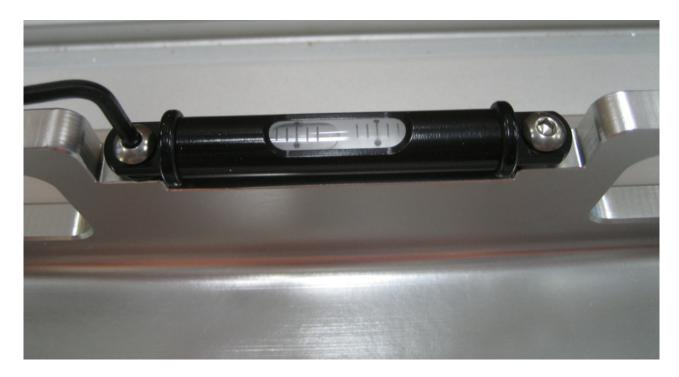
5) It was estimated to be four marks on the vial off-center. So you would adjust the screw to bring it back to two-off the original reading (again, camera angle makes it appear slightly to the left).
