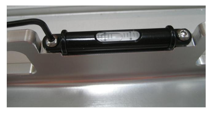
6) Now you can spin the LTW level and verify that the reading, whether it is exactly centered or not, is the same in either direction. You can now raise/lower the shim stack to establish a specific thickness to reset the level in the future. If you know it takes .012" on the right hand side, it makes it very easy to adjust the vial back to level at any given point in time, as long as your "reference" surface hasn't changed.
