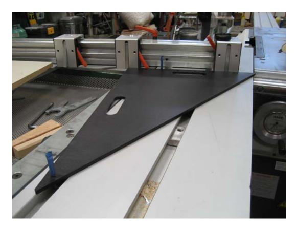
The above method is a bit fussy, you need to keep sliding the square back to the fence as you adjust, and use feeler gages to make sure both sides are touch the fence.. but it can be done.
