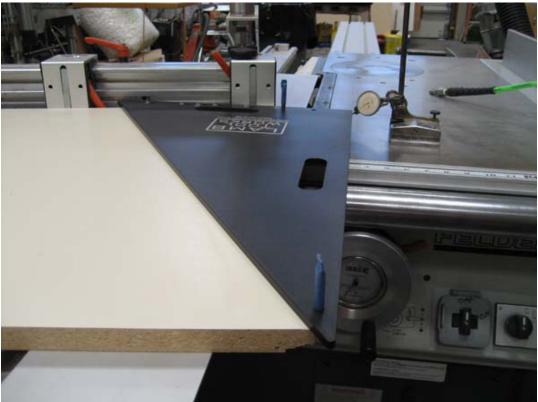
Again, set the indicator to zero and sweep from end to end. Adjust your fence, or the stops as required to get the angle correct.
