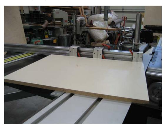
I have set the fence at 10° to demonstrate. Using the square, and two dowel pins (or 1/4" router bits with tape wrapped around the ends to prevent them from falling through the holes), set the square along the edge of the board with the pins in the corresponding 10° angle hole.
