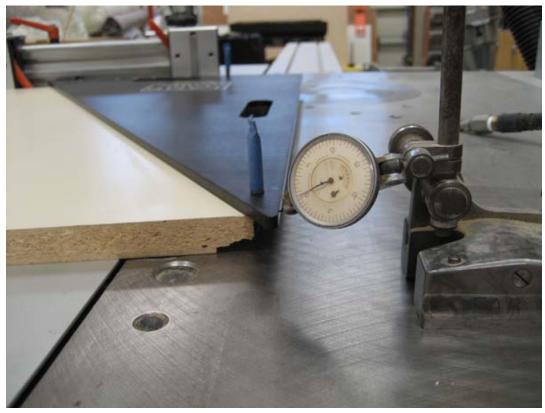
You can also use the square off of the slots in the slider.... if they run pretty true to the travel of the slider. You can hang your indicator out and indicate in on the slot, if it's pretty good then this is another way to set the angle. Flip the square over, drop the pins into the corresponding holes and then resting the pins snug against one side of the t-slot or the other, move it forward to the fence and you should hit the stops (or the fence) and be able to check/set your angle that way.
