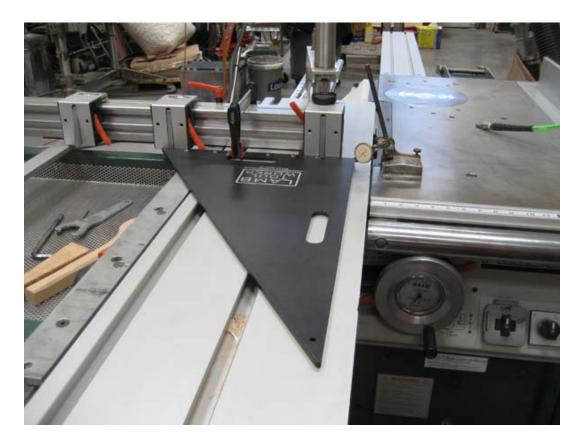
Then sweep from end to end, adjusting your fence stop as necessary to get the readings as close as you want at each end.
