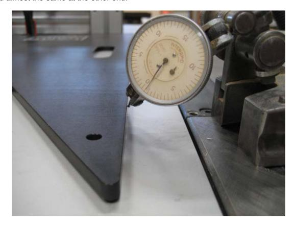
Now to check angles of the cross cut fence, I find it best to cut a large square/rectangle of material at exactly  $90^{\circ}$ , given you just set that, it should be easy.
