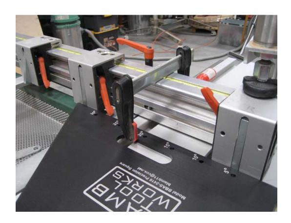
Next we place the test indicator and stand such that the needle can be zero'd against the 24" edge of the square. You might want to place a piece of 3/4" material under the square to lift it up, makes it easier to get a clamp on it.
