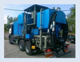
CUSTMAN 001072 Single cementing unit is suitable for a variety of fluid pumping and mixing operations in the oilfield. Typical operations include well cementing, well acidizing treatments, hydro-jet perforating, solvent pumping, pressure testing and miscellaneous fluid pumping at large range of Density (Range 9 - 19 PPG / 1,078 - $2,276 \text{ kg/cm}^2$  and flow rate (Range 1 – 7 BPM / 0 – 0.83 m<sup>3</sup>/min.
