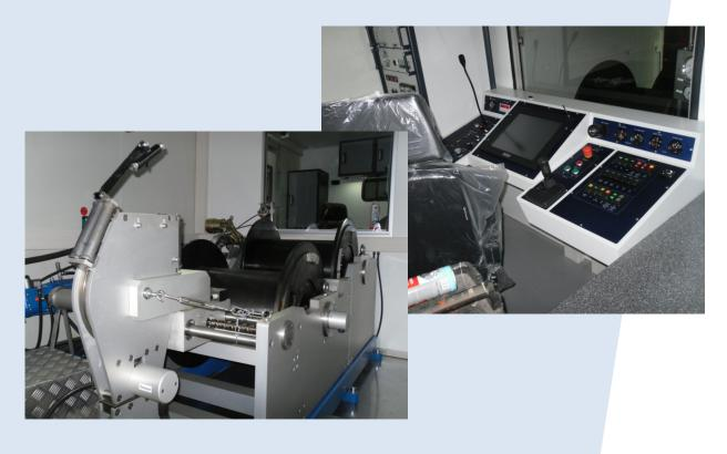
**LANDLINE "C" Slickline Unit** is designed for super light duty (.092") to super heavy duty (.125") slickline operations.
