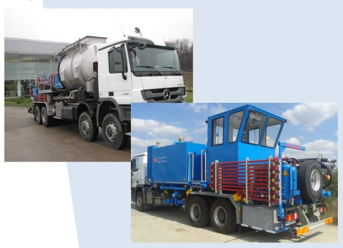
Acid Tanker, truck mounted, 8,000 liters capacity
