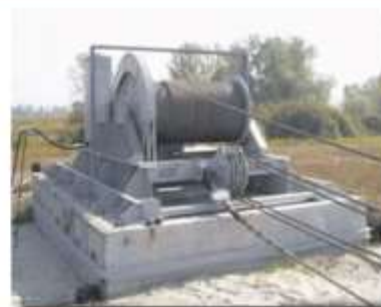
Rope winch with pulling force 80 t
