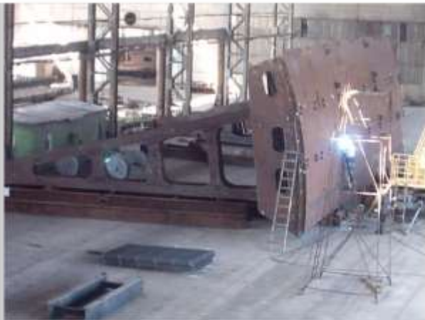
(The control assembly gate segment for Polotsk hydropower, Belarus, 2013)
