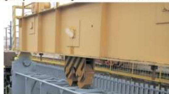
One-clamping devices lifting beam
