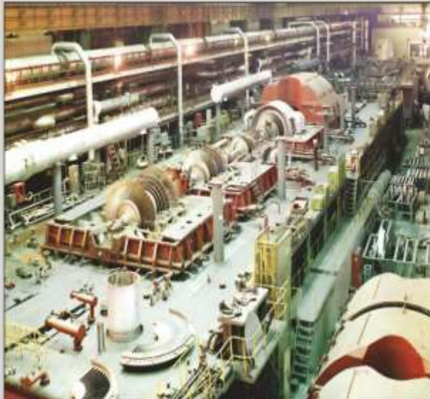
Assembly of steam turbine K-300-65-3000 on the works test bench
