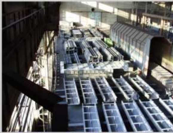
(Embedded parts of plain slide gates for Polotsk hydropower, Belarus, 2013)
