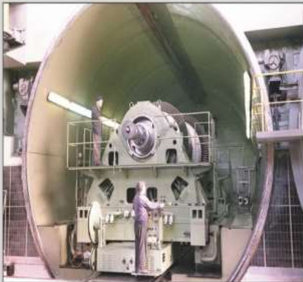
Balancing stand for steam turbine rotors
