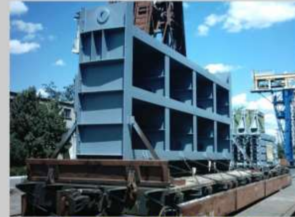
(Shipment section of plain sliding gate for the Nizhnegorodskaya HPP, Russia, 2013 )
