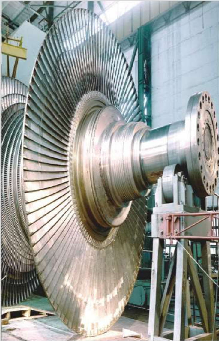
1000 MW turbine rotor of Zaporozhskaya NPP
