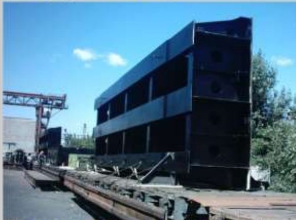
(Shipment section of plain sliding gate for the Kama HPP, Russia, 2013 )
