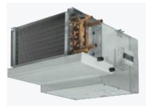
New "H Series" - High static units from 400 CFM up to 2200 CFM. Designed for jobs where high static pressure (0.50" max) is required. DX, Chiiled Water, Hot Water and Steam Coil options.
