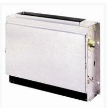
**HVWD/HVWS** - The cabinet is made of cold-rolled steel, phosphate conversion-coated then painted in a soft-white powder coated epoxy. This unit is for free-blow exposed wall mounting. The front panel is easily removed for complete service access. Unit also features a 4 way discharge grills for customized air discharge. Use VWS for sloped top units.
