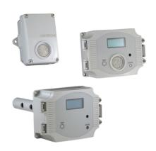
The AZ-CMD Series carbon monoxide detector uses an electrochemical sensor to monitor the carbon monoxide level and outputs a field-selectable 4-20 mA , 0-5 or 0-10 Vdc. The sensing range and output may be scaled to either 100, 150, 300, 400 or 500 ppm via the on-board menu. A front panel LCD is standard to ensure easy setup and operation. It is available in either wall/surface or duct mount configurations.
